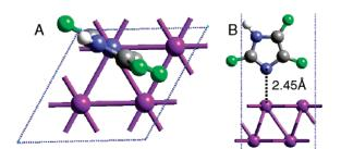
**Figure 1.** QM optimized structure of 2,4,5-trifluoroimidazole on Pt. (A) Top view of the periodic cell. The lower layer of Pt is hidden. (B) Side view. ImF3 binds through N to a top position in the Pt surface.
