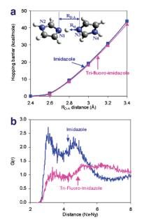
Figure 2. (a) Barriers for the proton transfer between Im/ImH<sup>+</sup> (blue) and ImF3/ImF3H<sup>+</sup> (magenta) in a dielectric with  $\epsilon = 23$  at representative donor/ acceptor N-N distances. The hopping barriers differ by less than 0.9 kcal/ mol. (b). Radial distribution function g(r) between donor and acceptor N sites of Im (blue) and ImF3 (magenta) Nafion membranes. The perfluorination decreases the number of close donor/acceptor neighbors.
